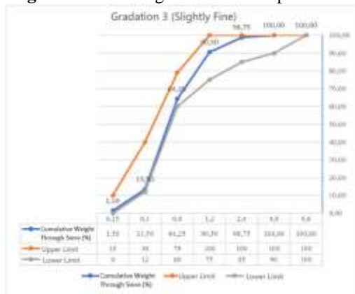
Fig 2. Gradation analysis graph of fine aggregate composed of moderately fine sand
