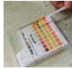
Fig3: The results of a litmus paper pH test
